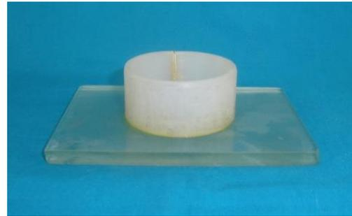
Figure 1: PVC cylinders were fixed on glass slabs by sticky waxed on glass slabs by sticky wax
